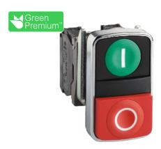
Harmony XB4, Double-headed push button, metal, Ø22, 1 green flush marked I + 1 red projecting marked O, 1 NO + 1 NC
