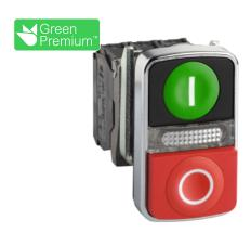
Harmony XB4, Illuminated double-headed push button, metal, Ø22, 1 green flush I + 1 pilot light + 1 red projecting O, 240 V AC, 1 NO + 1 NC
