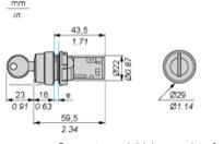
Support panel thickness: 1 to 6 mm/0.4 to 0.24 in. (metal), 2 to 6 mm/0.8 to 0.24 in. (plastic).
