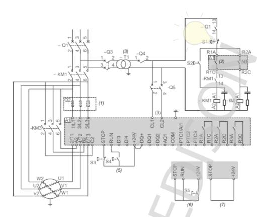
Connection inside the delta, with line and bypass contactor, type 1 and 2 coordination, non reversing, 2 wire or 3 wire
