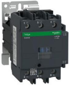
IEC contactor, TeSys Deca, nonreversing, 80A, 60HP at 480VAC, up to 100kA SCCR, 3 phase, 3 NO, 24VDC coil, open style
