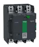
High power contactor, TeSys Giga, 3 pole (3NO), AC-3 <=440V 630A, standard version, 100...250V wide band AC/DC coil
